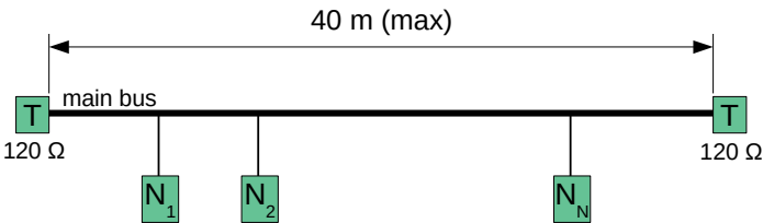
Figure 24: CAN line/bus topology principle used by Kanardia
