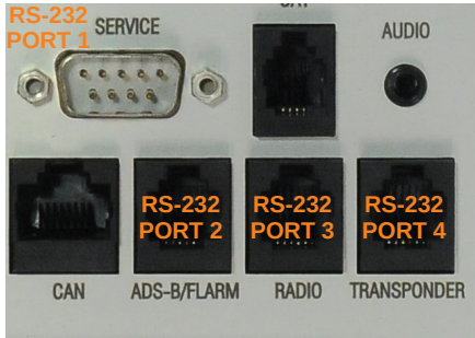
Figure 35: RS-232 ports at the back side of the Nesis.
