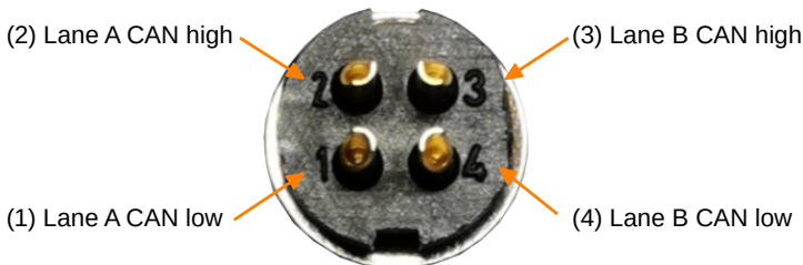
Figure 39: Cable plug back side. Note the four small numbers, which define the pin positions inside the plug. This is Binder part number 99 0979 100 04.
