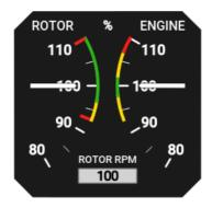
Figure 23: The combination of rotor RPM and engine RPM. Both scales are in percentages.
