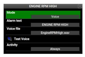
Figure 73: An example of alarm editor for the high engine RPM situation.
