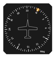
Figure 27: Illustration of the direction indicator.
