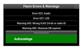
Figure 47: Left: a part of the main map screen, which shows the Flarm device status rectangle. Right: Flarm Error and Warning window. On top errors and warnings are displayed and the *Acknowledge* command at the bottom.
