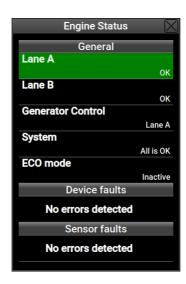
Figure 50: Detailed status information for Rotax iS engines.
