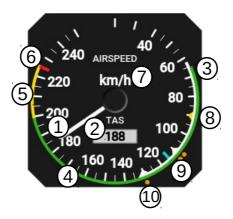
Figure 18: An airspeed indicator example optimized for an aeroplane using two step landing flaps.
