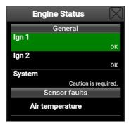
Figure 52: A more detailed status information for ULPower engines.
