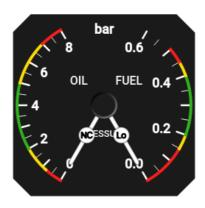
Figure 28: Round pressure indicator, with special markings shown on needles.
