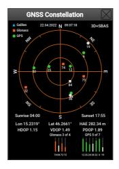
Figure 82: An example of GNSS details. The example shows bad satellite distribution and relatively weak signals.
