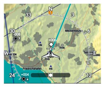
Figure 43: Traffic symbols on a map. Vertical difference is in hundreds of feet, as three digits are used.
