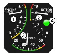
Figure 22: Four in one: the combination of engine RPM, rotor RPM, manifold pressure and prerotation helper lamp.
