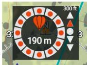
Figure 45: Left: Alert for an airplane, 330 meters away, slightly from right, 400 feet above and 10°- 30° above the horizon. Right: Alert for a balloon, 190 meters away, direction is not known, 300 feet above and 10°- 30° above the horizon.
