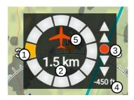
Figure 44: Threat classified as warning comes from left, distance is 1.5 km, about at the same visual level, 450 feet below.
