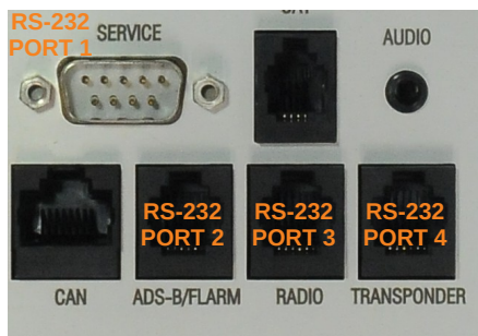
Figure 3.15: RS-232 ports at the back side of the Aetos.
