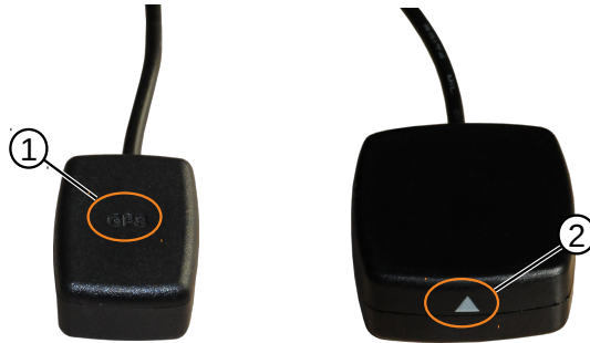
Figure 2.13: GNSS antenna orientation: ① – small, pure GPS antenna – the GPS text must be facing upwards, towards the sky. ② – larger combined GPS/Glonass antenna – the triangle must point upwards, towards the sky.
