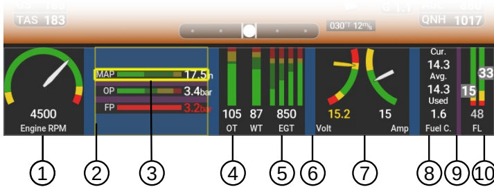
Figure 6.5: Illustration of main items used for editing the bottom part of the screen. Not all possibilities are shown.
