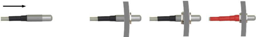
Figure 15: Inserting the OAT probe (left), cap is in place, tighten the internal nut, slide the insulation shrink sleeve (right).
