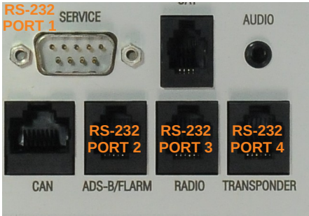
Figure 34: RS-232 ports at the back side of the Nesis.
