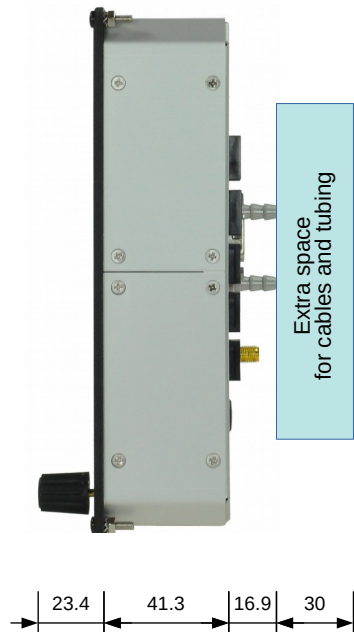
Figure 1: Nesis side view with dimensions.
