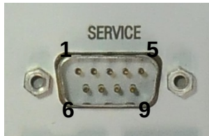
Figure 28: Service port D-SUB male with designated pins.
