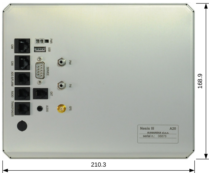
Figure 2: Back view with dimensions.
