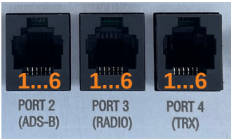
Figure 35: RS-232 ports with RJ12 connectors and their pin numbers.
