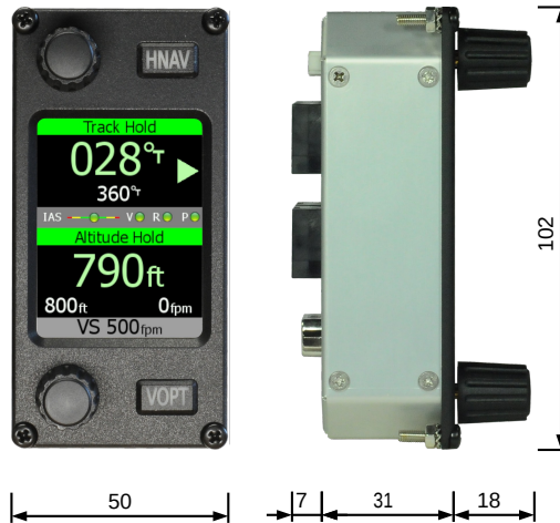
Figure 1: Front and side view of the Amigo with its principal dimensions. Dimensions are given in mm. Figure is not in scale!
