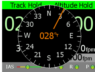
Figure 4: Navigation rose is shown for more intuitive track selection. Current track points upwards and orange needle points to a new track selection.
