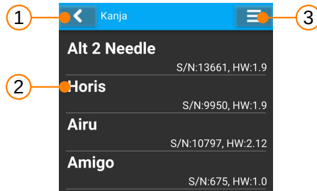
Figure 6: An example of devices detected on the CAN bus network.
