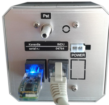
Figure 3: Blu inserted into an Indu device into one of the CAN ports.
