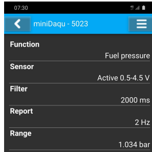
Figure 19: An example of fuel pressure sensor configuration.
