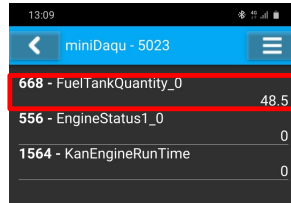
Figure 28: Checking tank indication value on the bus. Fuel level 1 is identified as FuelTankQuantity_0 . Value on the bus is always shown in liters.
