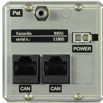
Figure 4: Back view of the 57 mm instrument with connections.
