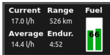
Figure 59: Fuel computer displays fuel economy, fuel level, endurance and range.
