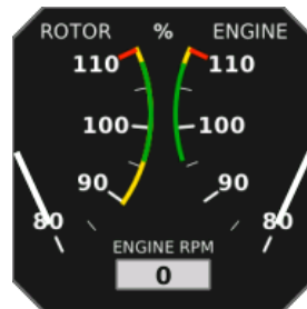
Figure 56: The combination of rotor RPM and engine RPM. Both scales are in percentages.
